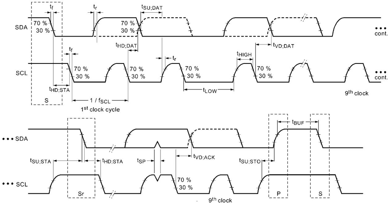
Figure 5. I<sup>2</sup>C Slave Timing Diagram
