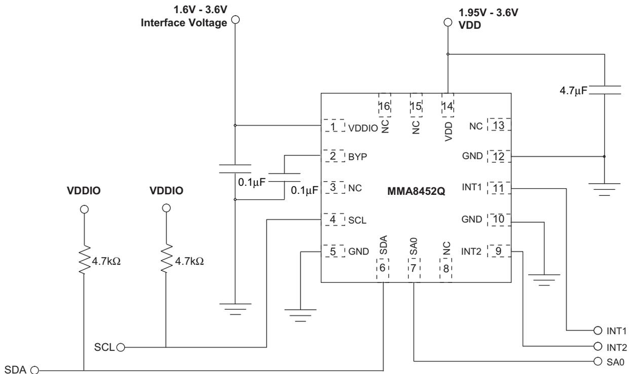
Figure 4. Application Diagram
