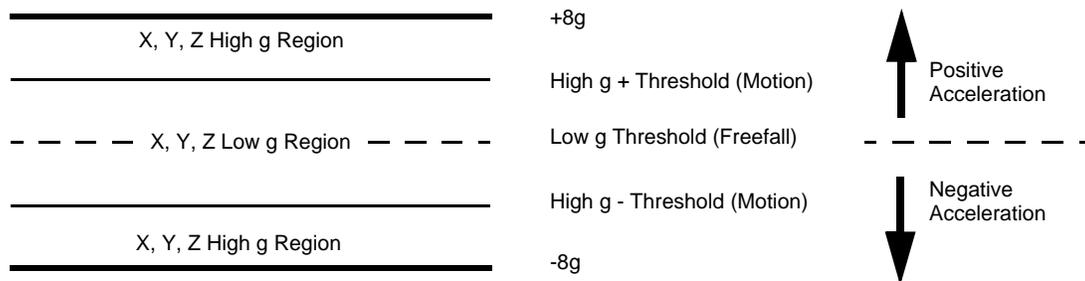
**Figure 13. FF\_MT\_CFG High and Low g Level**
