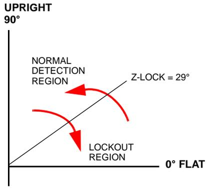
Figure 10. Illustration of Z-Tilt Angle Lockout Transition
