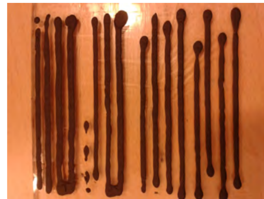
Figure 2: Conductive lines by the Fab@Home
