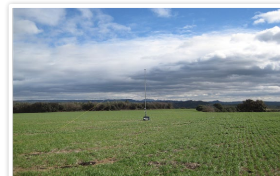
Fig. 8: The automated measurement receiver system on a flat terrain at 700 meters above sea level near St. Marti de Sesguiolles. The Montserrat Mountains can be seen at the horizon, Barcelona is behind them. Radio noise level is very low at this location.
