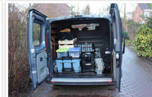
Fig. 7: Hired van with 8 antenna masts, 16 antennas, 32 of guy wires, 64 ground pins, 8 beacon transmitters, 10 batteries, 2 measurement receivers, and 2 tool sets.
