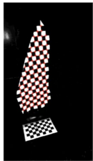
Figure 8: The high-contrast video frames (left). The 2D locations of the checkerboard corners in each video frame can be triangulated to obtain 3D coordinates (right). All 3D coordinates in all video frames will together form a digital reconstruction of the wing beat.
